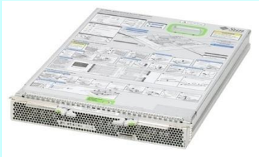
2+2 x Sun Blade x6440 Server 4 X CPU 6 Core AMD Opteron 8431
