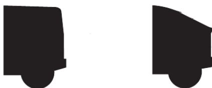
Fig. 5. Squareback and hatchback profiles
