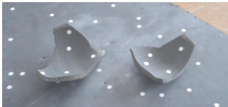
Fig. 2. Mobile laser scanning two elements of crockery, visible tags allowing to move the device relative to the objects.
