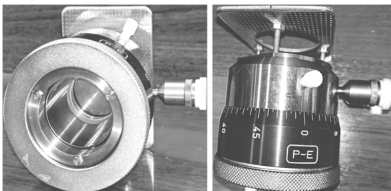
Fig. 1. Variable thickness KBr cell (Perkin-Elmer Inc.)
