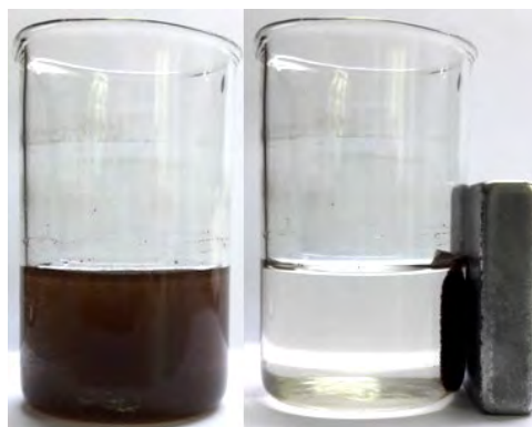
Figure 2: \text{Fe}_3\text{O}_4/\text{HPS} MN270 before and after magnetic separation.
