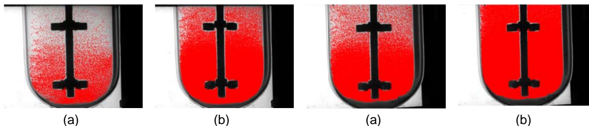
Fig. 3. Single bead detection after 30 min (a) and 360 min (b)
