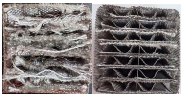
Fig. 1. Catalyst design with volume metal mesh (left) and corrugated and flat metal mesh (right)
