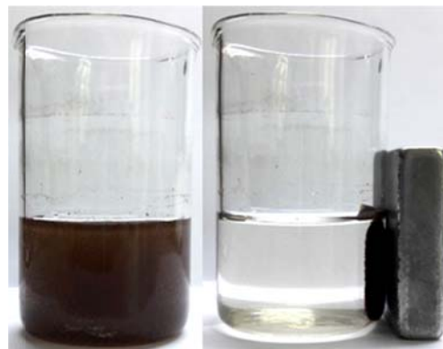
Figure 2. Fe 3 O 4 /HPS MN270 before and after magnetic separation
