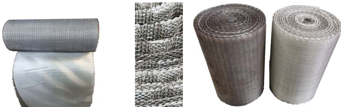
Fig. 2. The GFC-based structured catalytic cartridge
