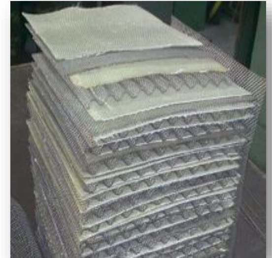
Packing with longitudinal arrangement of layers
