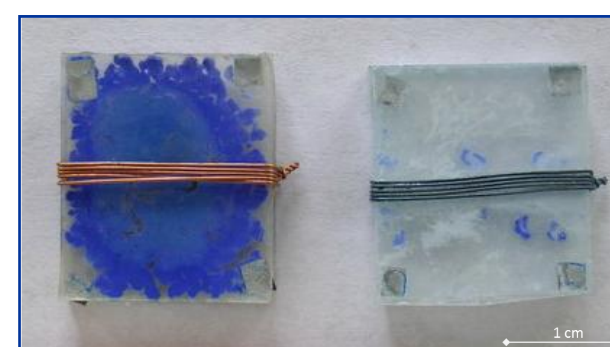
Samples after cleaning. 2A - after boiling in solution; 2B - after cleaning set-up.
