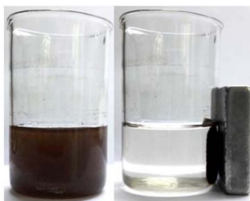
Figure 4: \text{Fe}_3\text{O}_4 /HPS MN270 before and after magnetic separation.
